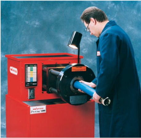
ProCrimp 1390 can be activated by foot pedal or hand operated switch.
